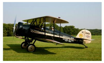
The only issue we had found with the airplane is the gear geometry. If you try to do a wheels landing, the gear splits, and, when it does, the airplane tends to go in any direction, making it a handful to control. So this airplane has to be three pointed to get some measure of stability upon landing.
