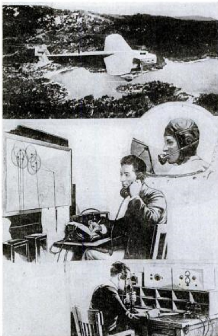
TOP—This transport plane is flying along a radio "track" that guides it to its destination. IN CIRCLE—Pilot talking to the supervisor. LEFT CENTER—The supervisor directs the planes and provides them data from the weather maps. BOTTOM—The station transmitter.
