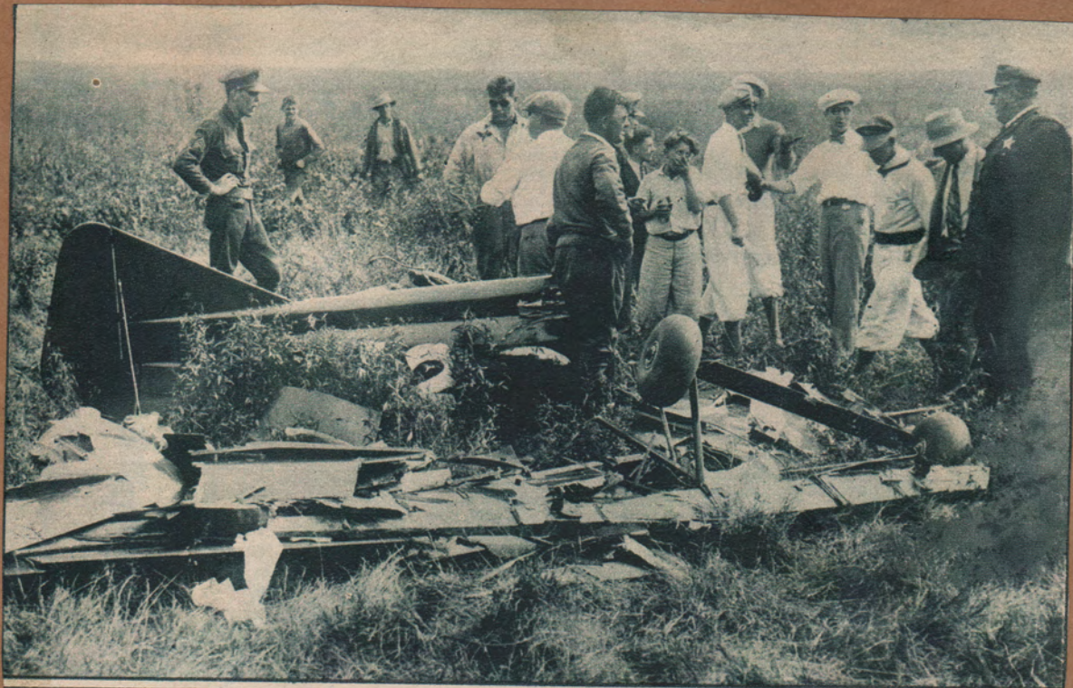
AFTER AN AIR RACER CRASHED AT THREE MILES A MINUTE: WRECKAGE OF MAJOR JOHN A. MACREADY'S PLANE. Which Was Scattered Over a Wide Area When One of the Wings Broke While the Famous Army Flier Was Leading in a Chicago Racing Event. He Was Seriously Injured But Is Expected to Recover.
