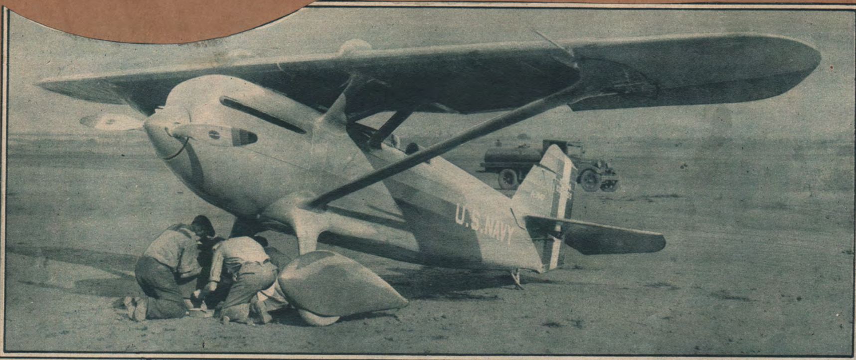
THE NAVY'S CONTENDER FOR SPEED HONORS IN THE CHICAGO AIR RACES: THE SPECIAL SEAHAWK MONOPLANE, Carrying an 800 Horsepower Curtiss Conqueror Motor, Which Is Expected to Fly at a Rate of More Than 250 Miles an Hour in the Thompson Trophy Free-For-All. Its Pilot Is Captain Arthur H. Page of the Marine Corps, Who Won the Curtiss Marine Trophy Event in May.
