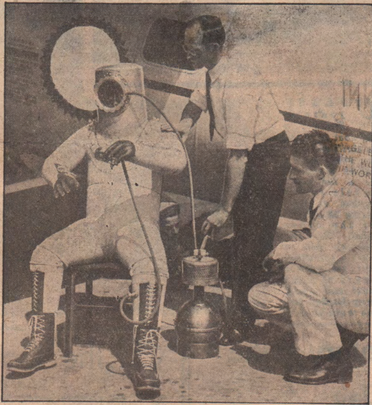
READY FOR STRATOSPHERE —Here is the stratosphere suit of Wiley Post, noted round-the-world flyer. Post was photographed in the suit in Chicago. Left is a closeup of the fur-lined outfit with aluminum helmet. Above is a demonstration of how oxygen is pumped into the tank that goes with the ensemble. (AP)
