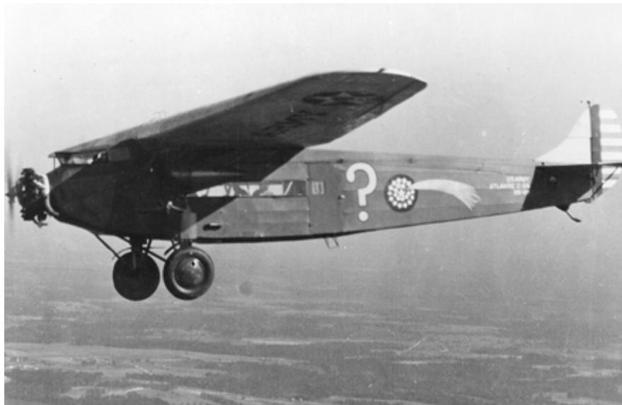
***Question Mark* was a specially modified Fokker C-2A sporting three powerful and fuel efficient 220-hp radial engines. Modifications included the addition of two 150-gallon fuel tanks as part of the new refueling system.**
