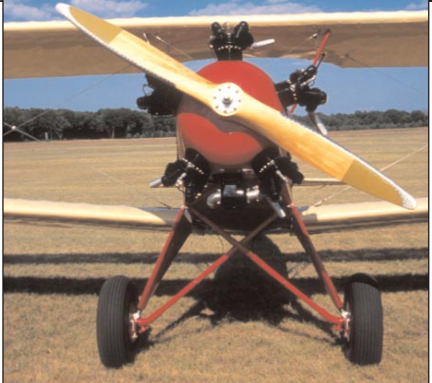
To make it less likely a student could nick a prop or scrape a wingtip, the Fleet was designed with plenty of ground clearance, thanks to a long landing gear. The compact size of the Fleet contrasts sharply with the much larger Stearman used for primary training a decade later.
