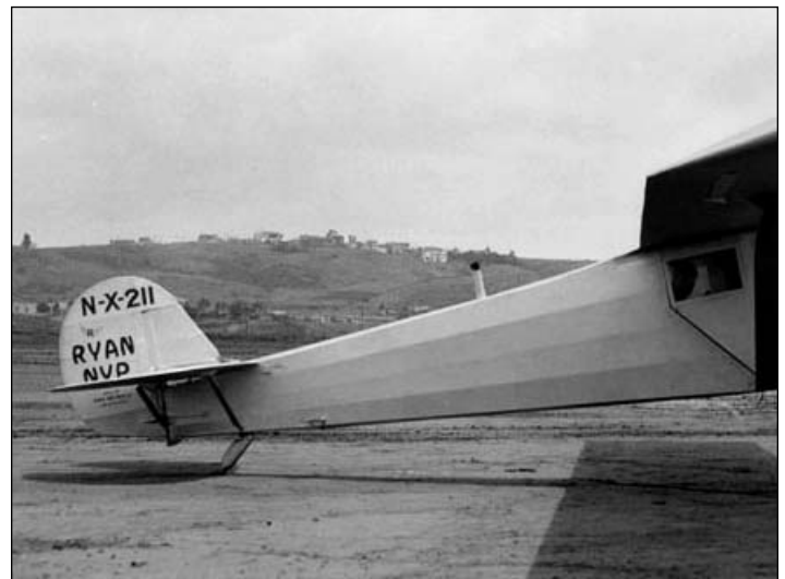
Charles Lindbergh's Spirit of St. Louis displays an X registration number on the Ryan NYP (New York - Paris) indicating that it was registered in the Experimental category in April 1927. As the aircraft was not a production design, the NX-211 registration would have been consistent with the regulations. The problem is that the use of X for Experimental was not officially adopted until 1929! (Photo from the Don Hall collection)
