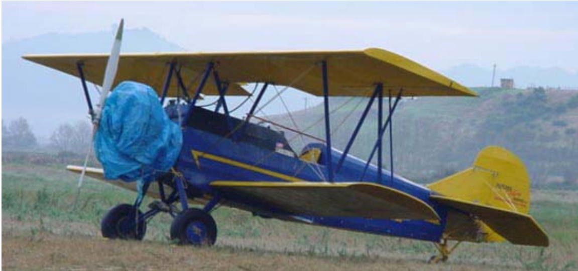
NOW: Mildred Morgan's NC8192 in New Zealand, fuselage hopper installed for agricultural dusting, and wings squared. Courtesy of Russ Ward.
