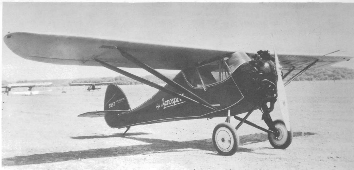
Fig. 159. Monosport model 1 with 110 H.P. Warner engine, had performance enough to delight anyone.
