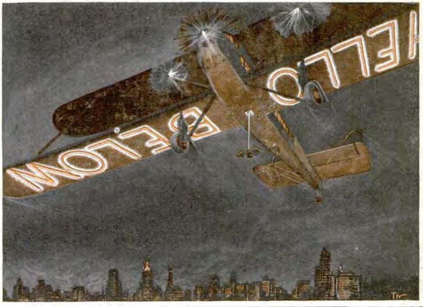
With an Enormously Extended Lower Wing, This Big Ship Has Carried a Neon Sign over Several Cities; Note the Cluster of Inspection Mirrors Projecting beneath the Fuselage
