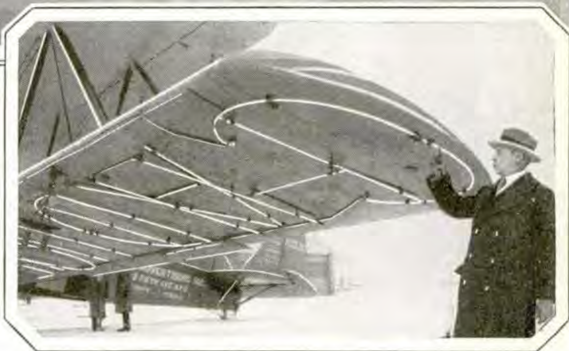
The Tri-Motored Bomber Rebuilt with an Enormous Lower Wing, to Carry the Neon Sign, and a Close-Up of the Glass Tubes
