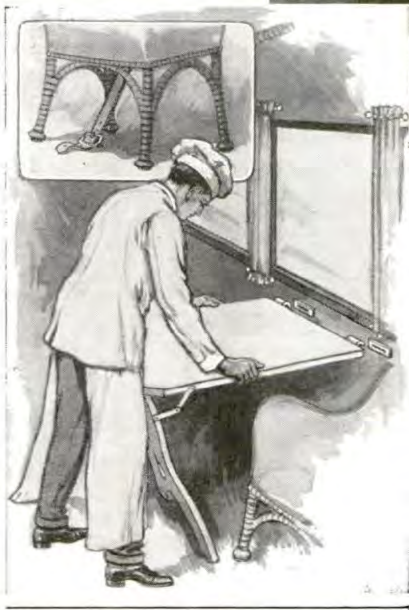
Dining in the Skies, and Sketch, Showing Method of Adjusting the Tables and the Chair Straps; the Plane Has a Permanent Desk for Writing
