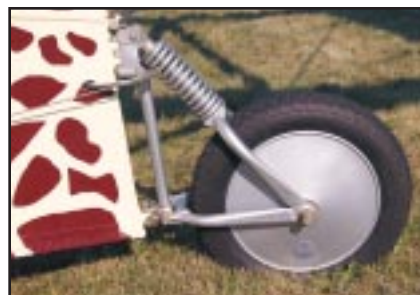
The large tail wheel also doubles as the water rudder.
