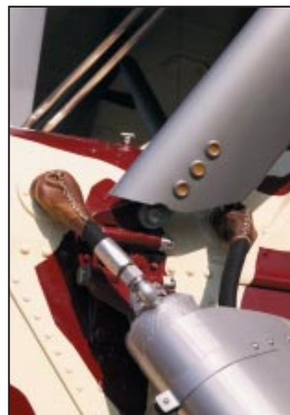
The large tail wheel also doubles as the water rudder.
