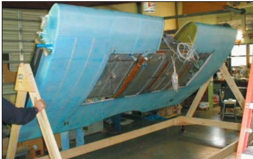
The completely new center section with its fabric covering applied. You can see the fuel tanks installed in the center section, which was done in the S-39C model of the airplane. Earlier versions had the fuel in tanks located in the hull.
