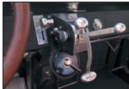
The engine control quadrant, like the control wheel, is original.
