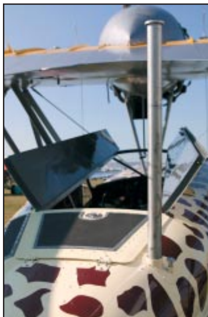
The two long hatches and the smaller aft hatch allow you to gain access to the cabin. The aluminum vertical tube is a retractable handle that makes the climb up easier.
