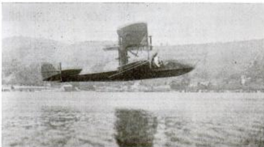
The first flying boat was invented and developed at the Hammondsport plant by Curtiss in 1911. Note that this first boat has no "step" in the hull. The step was a later development that made take-off easier.
