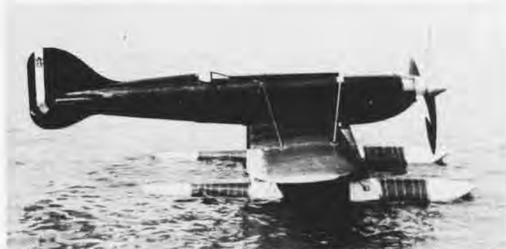
Bold Italian concepts found form in such unorthodox designs as the 1929 Piaggio P7, top, a combination boat and aircraft. Small rear propeller provided sufficient thrust for hydrofoil-finned fuselage nose to rise clear of water as 1,000 hp was applied to front propeller. Aircraft never flew. Macchi MC-72, below, attained 440 mph in October 1934 for world speed record.
