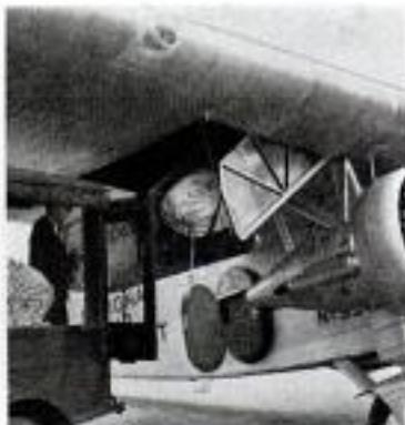
One addition to the old Tin Goose was this type of retractable mail compartment.
